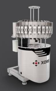
**For many concentrator plants.** Boxray 24 consists of a carousel equipped with 24 measurement cells that enable a single analyzer to monitor multiple steps in the process, from ore to concentrate. As each stream has its own loop and measurement cell, there is no risk that samples will be contaminated by other streams, which can corrupt analysis results.
