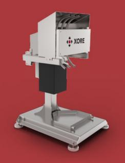
**For most concentrator plants.** Boxray Compact has three measurement cells that are mounted on a sled that moves sideways. Two of the cells are used for streams and the third is adapted for a reference sample. Boxray Compact is equipped with a multiplex system that allows up to 16 sample streams.
